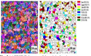
**Fig. 2 (a)** EBSD Euler map of the original grain structure, (b) texture component map[1]
