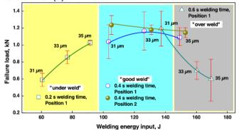
**Fig. 12**. Effects of welding parameters on the failure load and welding energy input.[6]
