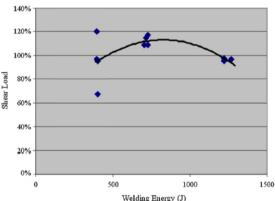
**Fig.8** The shear load (at the aaa|C interface) vs. ultrasonic welding energy for aaaCwelds.[4]
