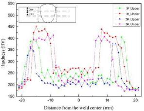
Fig. 6 Results of hardness measurements.[3]0.
