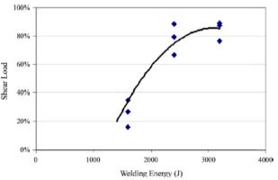
**Fig.7.** The shear load (at the ccc|C interface) vs. ultrasonic welding energy for cccCwelds. [4]
