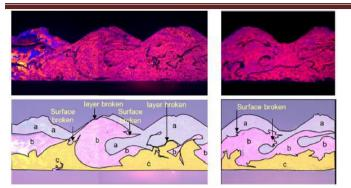
**Fig. 10** Sectioned and etched Al tabs interfaces, observed by OM (1.8% HBF4 in distilled water; 20 vdc for 2 min; sample at anodic pole; Olympus OMG 3; polarizinglight plus sensitive tint lens). Cu bus bar is not shown.[4]
