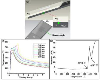
**Fig. 11**. Temperature at the weld interface: (a) measurement setup; (b) temperature history curve; (c) differential scanning calorimetry result of AZ31.[5]
