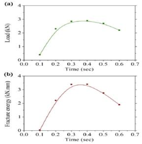
**Fig. 1 (a)** Average lap shear strength and (b) Failure energy with increasing welding time under a 1.4kN clamping force.[1]
