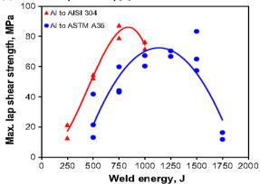
**Fig.3** Maximum tensile lap shear strength of dissimilar USWed Al 6061-T6-to-AISI304 stainless steel (a) and Al 6061-T6-to-ASTM A36 steel (b) Joints at different energy inputs [2]
